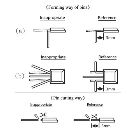
\* Recommend : Use metal mold to closely locked pins, and do not apply stress on black body of IC during processing. The ideal processing location of IC's pins is at least keeping 3 mm length.
